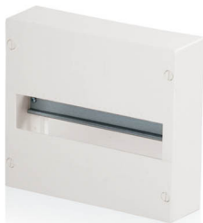
name N 12 A type IP 30 □ In 63A dimensions 250 x 225 x 70 number of modules 12 + 2 PE, N terminal 2 x 10
