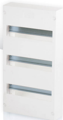
name N 36 A type IP 30 □ In 63A dimensions 250 x 463 x 70 number of modules 36 + 6 PE, N terminal 2 x 15
